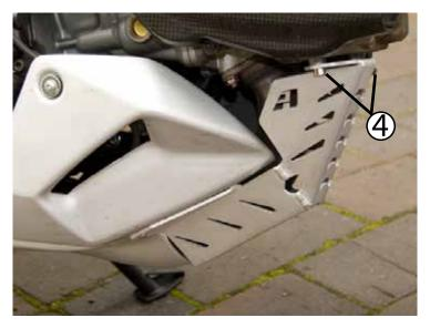
Using a 5mm allen tool, tighten the (2) M6 bolts down. Do not OVER tighten these.
