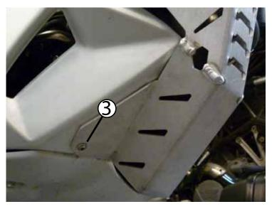
Using a 3mm allen tool, insert the M5 (provided) with M5 washer. Tighten this fastener down, do not OVER tighten.
