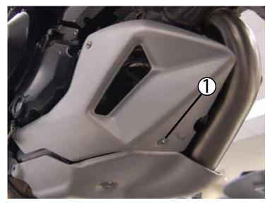
Using a 3mm allen tool, remove the OEM fastener.
