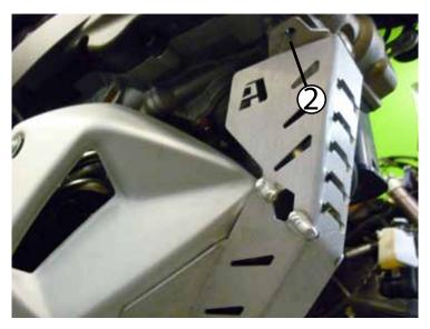
Apply thread locker to the last couple of threads on the (2) M6 cap head screws. Line up the Header guard as shown, and insert the M6s. Turn them a few turns for now.
